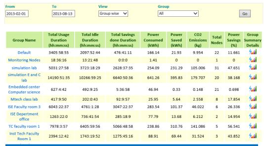
Hours of usage, idle times and energy consumption was rapidly discovered using IPMPlus
